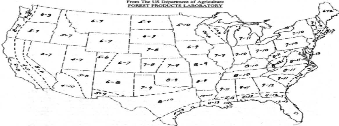
Variation of average moisture content. In each pair of figures, the first is average moisture content during January and the second is average moisture content during July for wood used indoors.
