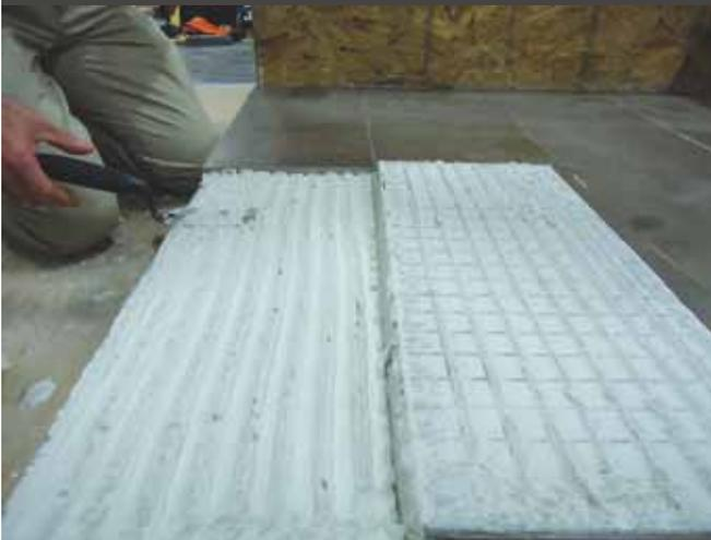
With the popularity of large-format tile continuing to grow comes the necessity of providing an adequate supply of thin-bed or medium-bed mortar to properly support and bond the tile. The question is, which trowel notch works best?
