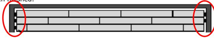
3. If the starting or ending wall is irregular, scribe or trace the contour of the wall to the row of boards.
